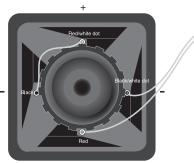
Dual 2 Ohm = 4 Ohm load Dual 4 Ohm = 8 Ohm load
